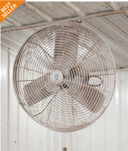
24" VES High-Velocity Single-Speed Circulation Fan Tapered intake and exhaust designed for optimum performance, maximum air velocity and distance coverage. Standard OSHA safety guards mean you can mount these fans at any height. Versatile wall and ceiling mount pivots 180°; fan can turn 360°. High efficiency motors are totally enclosed with sealed ball bearing. Well balanced, strong blade design for years of trouble-free service. Easy to clean. Includes 9' L power cord. 115V, 8,800 CFM. Can be converted to variable speed if switch is purchased separately, otherwise it will run on high. Switch available through special order. Allow extra delivery time. C35642V121
